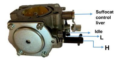
This is the standard carbohydrate. As an engine manufacturer, of course, any carburetor must be adjusted based on weather conditions and flight altitudes.
