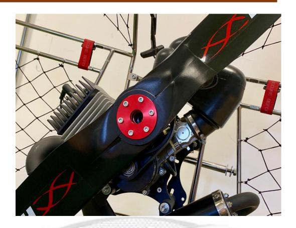
In the case of propeller impact, it is necessary to verify that all the engine parts have not suffered any damage, paying particular attention to the components listed below: Reduction pulley and bearings; Reduction eccentric; engine's crank case and crankshaft, crank case support and engine rubber mounts.
